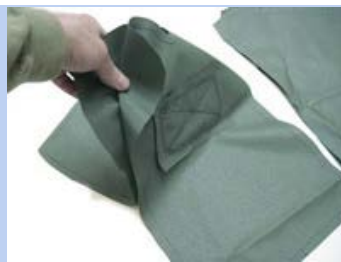
Two pieces joined front to front
