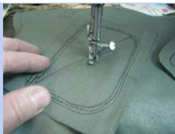
Stitch around the rectangle 3 times, then "X" across
