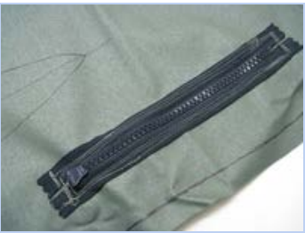
Stitch zipper 3 times around as shown here
