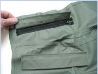
Finished zipper flaps sewn inside each zipper
